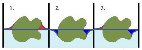
Blue: Increases amount of water displaced, stronger buoyant force Red: Decreases amount of water displaced, weaker buoyant force
